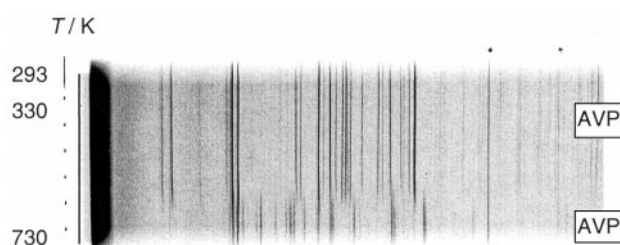
Fig. 9 Guinier-Lenné pattern ( Cu\text{-}K\alpha_1 ) of the phase transformation of AVP to AVP' under N_2 up to 730 K ( \beta=1\text{ K min}^{-1} ).
